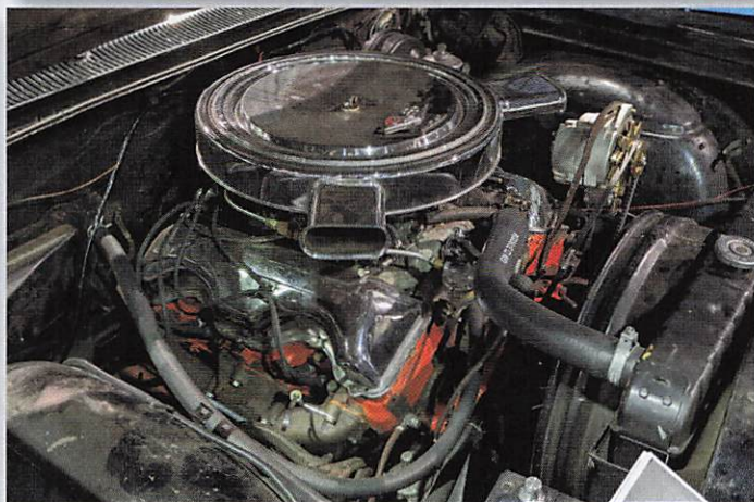
...a full-size Chevrolet X-frame chassis with a modified Pontiac body, an amalgam of Chevy and Pontiac interior components and in this case, a 409/425 Chevy V-8 hooked to a four-speed manual transmission. This is an incredibly rare machine and we hope it's returned to its former glory.
